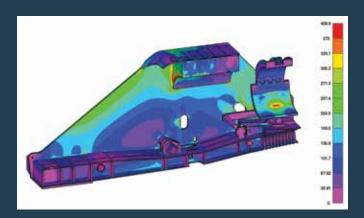
This model shows the stress calculation that Maats engineers carried out. As a result of these calculations, the engineers decided to use a high-strength-steel quality for the frame. With that high standard it leaves no doubt that the machines can bend the range of pipe specifications without any problems, also at low temperatures.
