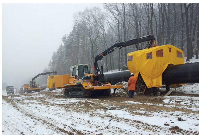
Figure 2. The SR714 Welding Tractor has optimal machine stability and all attachments remain fully operational on inclinations up to 45°, allowing the machine to optimally function in difficult mountainous areas.
