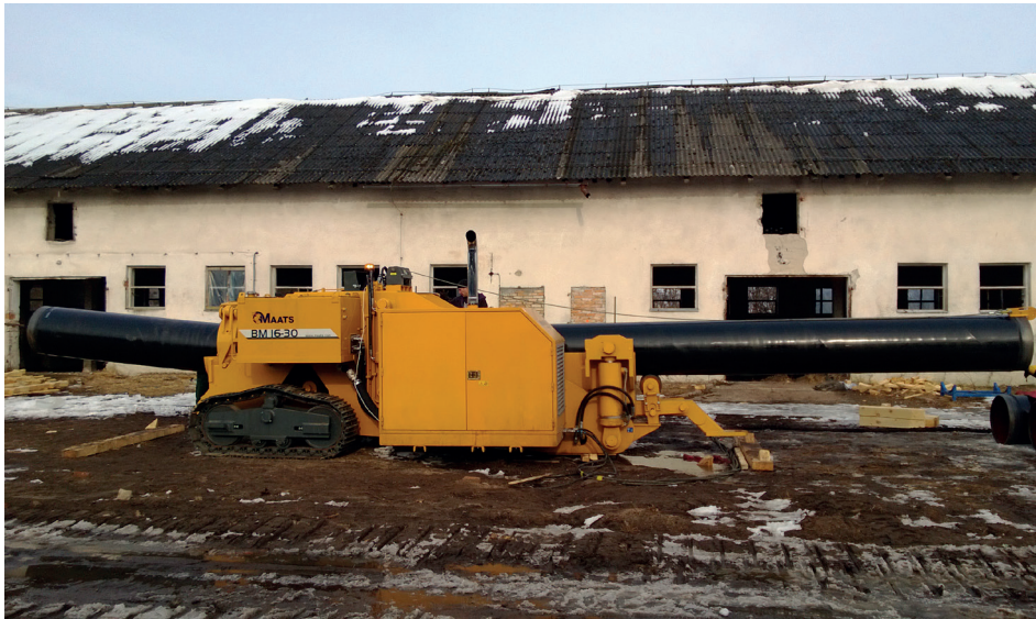
Figure 4. Prepared for extremes, the Maats bending machines can bend X100 steel pipe up to 1 in. wall thickness of the largest loadable pipe size. The specially developed frames allow the machines to even carry out work in arctic or tropic conditions without compromising its unique bending specs.
