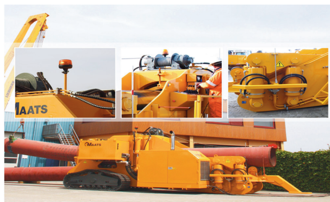
Figure 3. Maats bending equipment; The unique high strength of the construction is developed to withstand high bending forces and guarantee safe operation in all possible climates. The machine is equipped with numerous safety features and the layout is optimised for safety.
