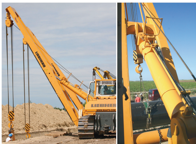
Figure 1. Boom and boom-cylinder, one of the 'hidden' but majorly important safety features on Liebherr and Maats pipelayers.
