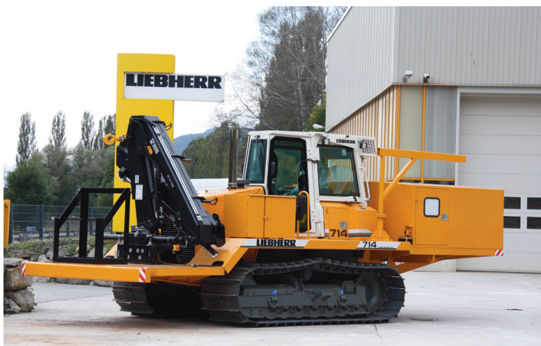
Figure 5. The Liebherr SR714 consists of numerous innovative solutions such as the fully hydraulic-driven concept, several emergency stop buttons, centrally located function controls and ROPS cabin with heater and air conditioning.
