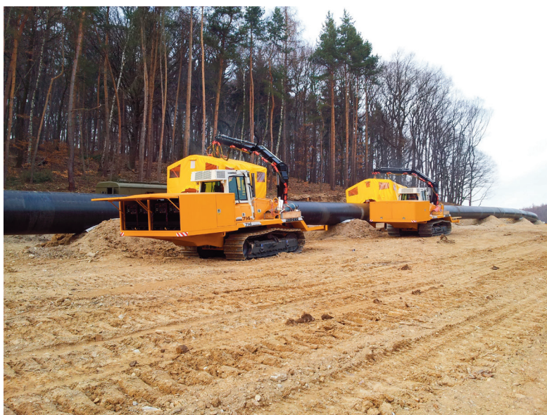
Figure 4. The Liebherr SR714 welding tractor has an extra long undercarriage, wide track shoes and extreme low centre of gravity, providing utmost stability and low ground pressure to guarantee safe operation and optimal use in all ground conditions.
