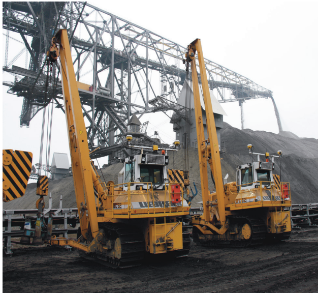
The previous model Liebherr RL52 conveyor belt shifters, complete with Trimble GPS antennae.
