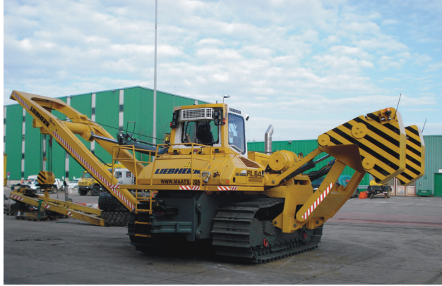
Machine prepared for operation. The machine features include a special boom, walkway, automatic drawbar coupling, cameras and beacons, as well as extra LED-lights.
