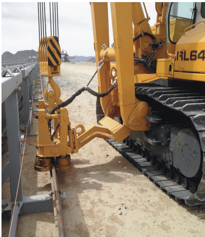
The hydraulic roller head is powered directly from a PTO on the machine.
