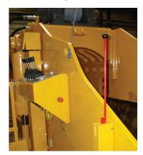
The safety lever is an extra safety feature on the Maats bending machines. The safety lever secures the machine from making any unintended movements.
