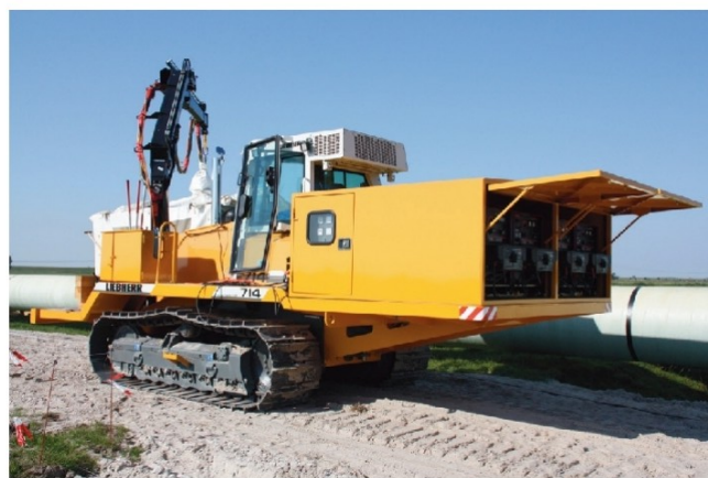
Figure 2. The lockable compartments on the SR714 provide easy, yet safe access to the generator, compressor, air tanks and welding equipment.
