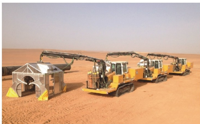
Figure 3. The extra long undercarriage, wide track shoes and extremely low centre of gravity offer the utmost stability and low ground pressure, guaranteeing optimal use and safe operation in all ground conditions.
