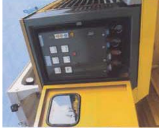
The electric generator is driven hydraulically for constant weld quality.
