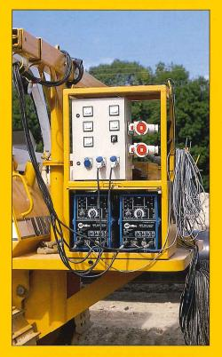
In order to be able to utilize the pipe layer as a universal machine for various tasks, a welding generator can be installed on the rear, and it is also driven by the standard working hydraulic system, with electronically monitored speed regulation. In addition, hydraulic drives for pipe facing machines or for a loading crane can be installed without any problems.
