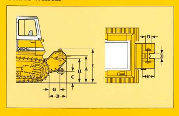
Pulling power, max.: Cable speed: 300 kN (30.6 t)/ 67,500 lb 0-96 m/min. (0-315 ft) stepless 22 mm (7/8") 50 m (164 ft) 1200 kg (2650 lb) Cable thickness: Cable length: Weight:
