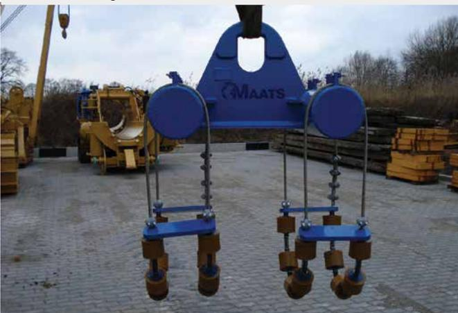
In addition to the roller cradle program, Maats also produces C-cradles for smaller pipe sizes (2-12 inch).
