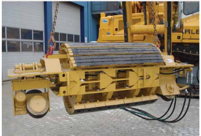
Based on your pipe specification the mandrels are set to the correct wall thickness and will be delivered to your jobsite "ready-to-use".
