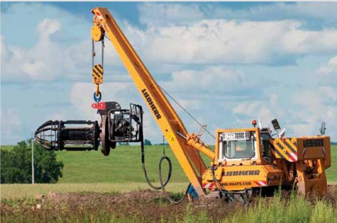
In case the pipe joints have to be machined to prepare them for welding, Maats can supply a pipe facing machine. Together with a hydraulic power unit, a pipe facing machine can be used to machine all common and most complex bevels. There is even the possibility to directly power a pipe facing machine from a hydraulic PTO on a Liebherr pipe layer.
