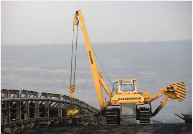
Based on the Liebherr pipe layer, Maats can supply a conveyor belt shifter. With several special options and the easy joystick operation, the operator can keep his eyes on the conveyor belt in order to keep the risk of fracturing the rail to a minimum.
