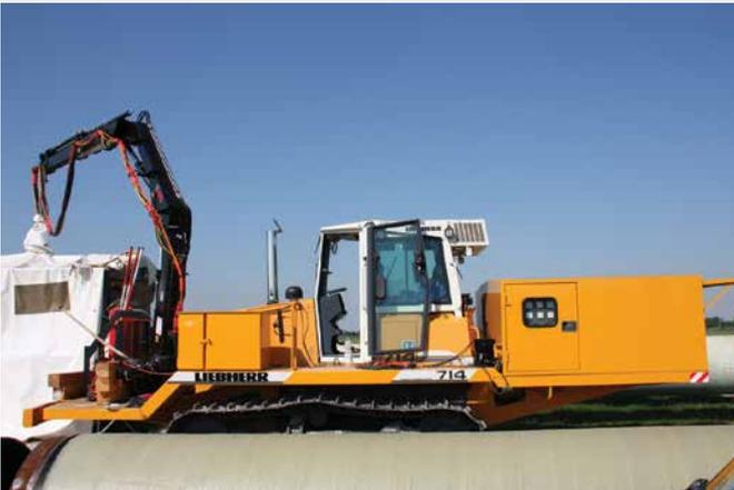
Together with Liebherr, Maats has developed two different sizes Liebherr welding tractors. The Liebherr welding tractors / paywelders can be equipped with up to six welding sources. These welding sources are driven by a hydraulically powered generator with a standard capacity of 140 kVA (other capacities available). The generator is powered directly by the main engine of the welding tractor. As an option, a hydraulically powered compressor can be installed.
