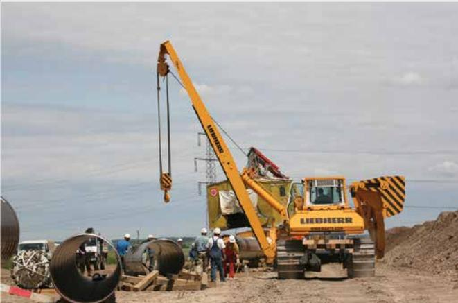
All machines feature the characteristic Liebherr hydrostatic drive and all new machine types are equipped with a fully enclosed cabin with ROPS structure as a standard. This provides a safe and conditioned working environment for the operator, making Liebherr pipe layers the safest and most reliable pipe layers currently available in the market.
