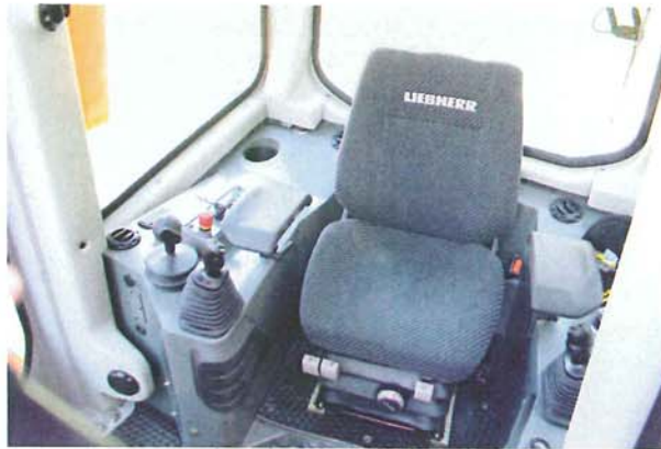
Figure 3. Fully enclosed cabin with 15° turned seat.
