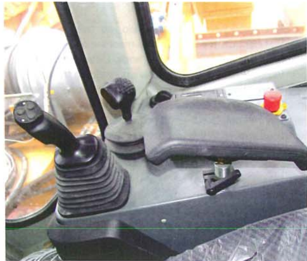
Figure 5. Single joystick operation.
